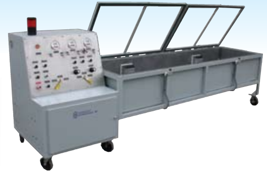
Tube & hose test stand rated to 30,000 PSI fully automated.
