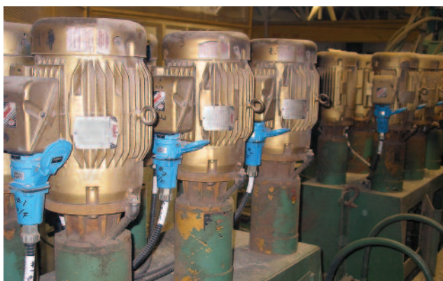
Decontactors enable quick motor change-outs
