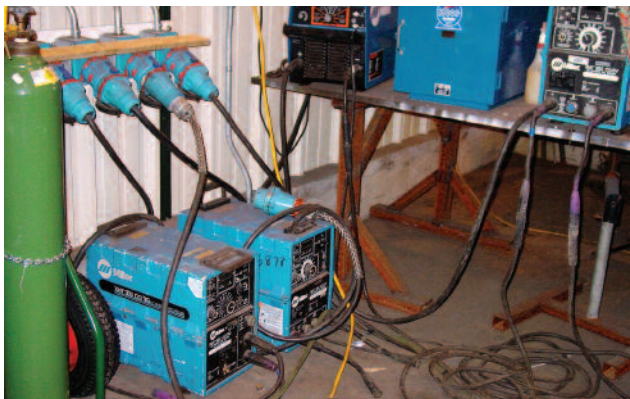
Decontactors allow welders and other equipment to be safely connected and disconnected, even in overload conditions.
