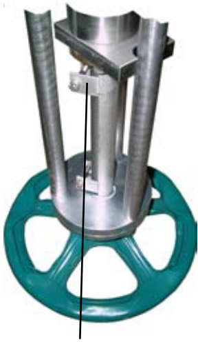
Arrangement A Special half pipe blocks the stem within top works and prevents valve from stroking
