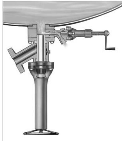
Fig. 2 - Drain Valve Open for Sample
